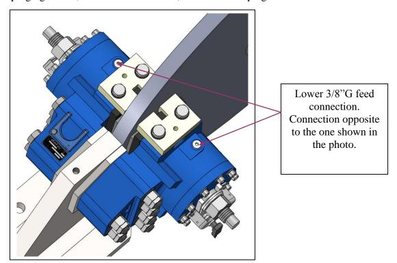
2.3.7. After fitting the hydraulic connections, apply 2 Mpa of pressure to the brake to bleed the air out of it. The purging of air out of the 3/8"G hole is done without hydraulic feed. In the event of not having the option of fitting a minimex outlet, the brake air can be bled out through the upper feed connection, by unscrewing the steel plug until oil comes out. At that time we will know that there is no longer any air in the brake, so we can screw the plug back on.
