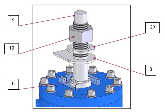
7.4- The block of springs is still compressed, so that if now the cover is removed (marked 3), the springs would exert a force that could be dangerous for the worker.
