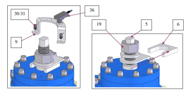
4.1.3 Adjust the adjustment screw (marked 5), by tightening or loosening until the distance between the lining and the disc is of 1 mm. We will refer to this distance as the air gap. Important, measure this distance using gauges.
