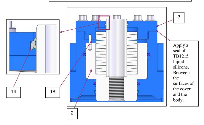
7.17- Proceed with the procedure described in point 2 (brake assembly procedure) and in point 4 of the instructions (adjustment of the brake).
