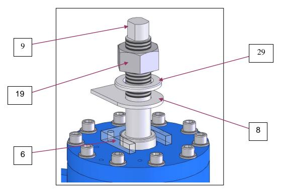
6.4- The block of springs is still compressed, so that if now the cover is removed (marked 3), the springs would exert a force that could be dangerous for the worker.
