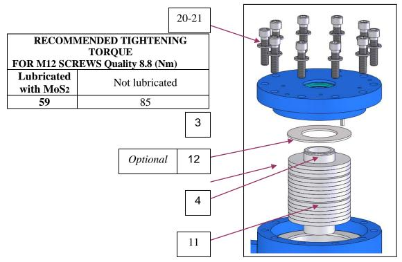
6.8- Fit the spring guide (marked 4) into its place taking care to fit it into its lodging of the piston (marked 2).
