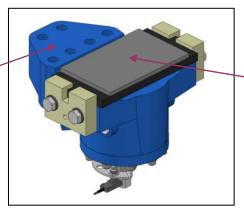
Contact surface between the linings and the disc.
